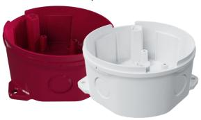
TFA-0130 Deep base is used to allow cable tube entry and cable connections to be made easily on the detector base, especially where surface mounting is performed. Deep base can be used for all Teknim detectors and sounders and can also be used with TFA-0135 Base heater.
