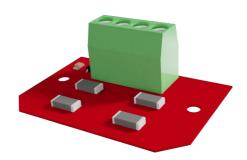
The TFA-0135 is a heater that must be installed inside the TFA-0130 Deep base and is used to raise the temperature of the base. It is intended for use in environmental conditions where freezing or condensation can occur on the detector base, potentially leading to false alarms. Its purpose is to raise the temperature of the connected detector by a few degrees, thus preventing issues caused by condensation in the sensing chamber or on the electronics.
